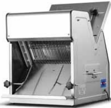
Bread Slicer (SS) Size: 760×560×780mm Power: 370W Thickness of Slice: 12mm No of Slice: 31
