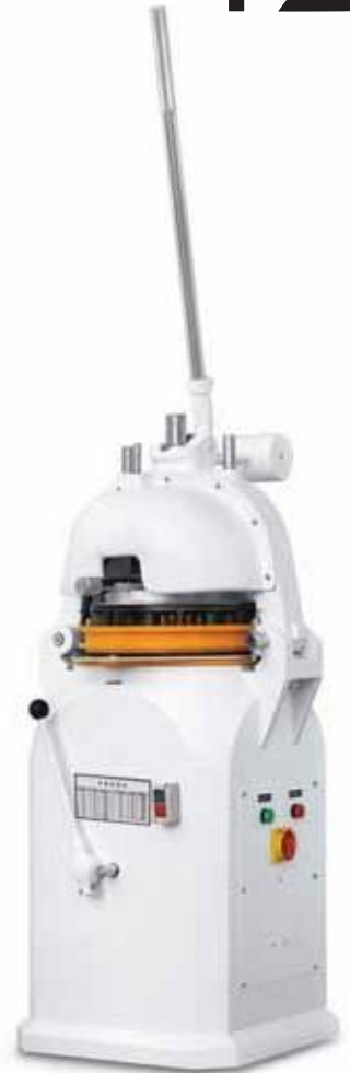
Dough Rounder Divider Size: 640×540×2100mm Power: 750W Dough Weight: 30~100gm
