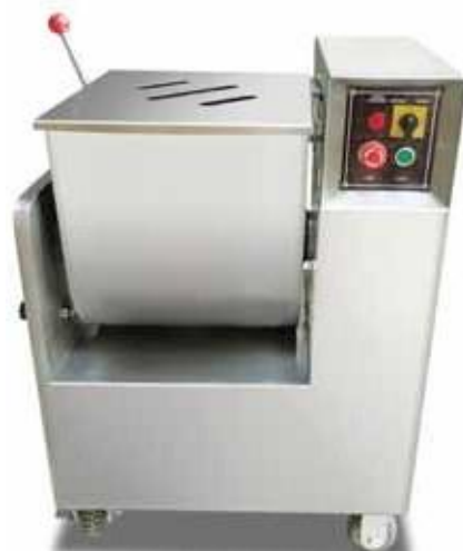
Filling Mixer Size: 670×510×1100mm Power: 0.75Kw
